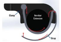
7. Tighten both mounting clamp screws to 35 in lbs (4.0 Nm).
