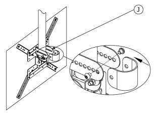
7. ATTACH SAFETY TETHER Vision projector mounts include a safety tether which should be used to attach the flat-panel to the base of the mount pole.
