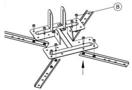
3. ATTACH BRACKET ASSEMBLY TO FLAT PANEL Ensure four screws are used for safety.
