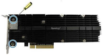
**b** Tighten the full-height bracket with two screws.
