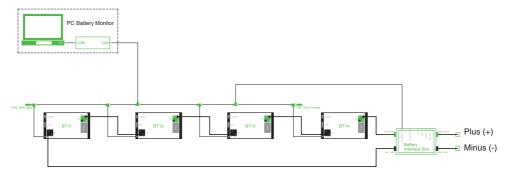
Figure 5. CAN Bus network topology
