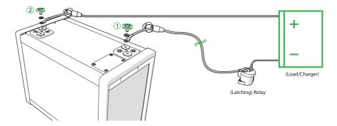
Figure 7. Connecting the battery to the load
