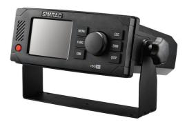
The V5035 consists of a transceiver radio unit, an integrated GPS receiver, a controller unit, and a color 3.5" LCD display with menu keypads. The radio has three receivers -- two TDMA receivers and one DSC receiver. The transmitter alternates its transmission between the two operating TDMA. The controller unit creates and schedules data packets (containing dynamic, static and voyage related data) for transmission based on the IMO performance standard for AIS.
