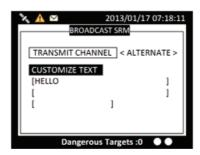
To save entered text, press and hold the knob for 2 seconds.
