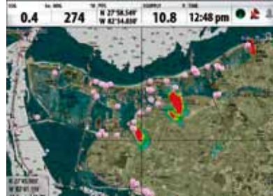
Broadband 4G Radar shows three individual rain cells inside the storm pictured on the left > 17nm away
