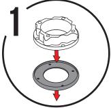
Place the plastic base onto the rubber base gasket. Be sure to line up the four screw holes.
