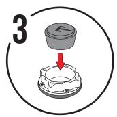
Insert the rubber gromet into the plastic base.
