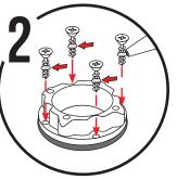
Apply some marine sealant to the threads of the screws. Screw in the four screws using a philips head screw driver.
