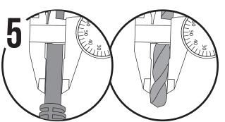
Measure your cable diameter and select the appropriate drill bit.
