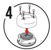
Line up the Cable Gland cover with the four holes in the plastic base and screw the bolts in with a allen wrench.
