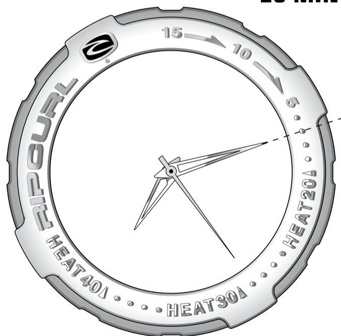
BEZEL INDICATING THREE MINUTES TO GO IN A 20 MIN HEAT
