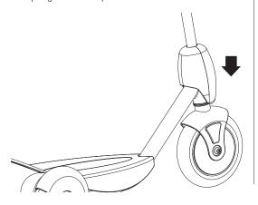
**6** Slide headset cover all the way down to cover collar clamp and connectors.
