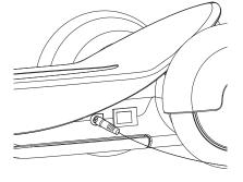
**2** Plug the charger into the charger port. The light on the charger should turn red during charging. The light on the charger will turn **OFF** when charging is completed.
