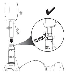
**3** Slide the headset cover up. Depress the spring loaded button on the T-bar and insert the T-bar into the front fork until the T-bar is securely locked into place.
