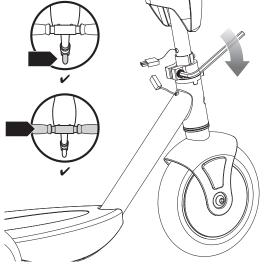
**4** With the front wheel pointed straight ahead, the handlebars square to the front wheel and the Razor logo on the T-bar facing the front, tighten the bolt on the collar clamp. Tighten securely.
