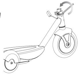
2 Loosen the 5 mm bolt on the collar clamp.
