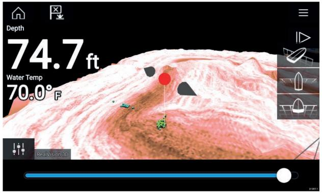
You can move the waypoint along its current axis by sliding 1 finger across the screen. You can also adjust the view onscreen using the usual 2 finger touch gestures.
