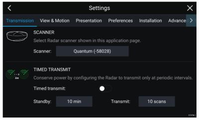
Select the Scanner: box on the Transmission tab. A list of available Radar scanners is displayed.
