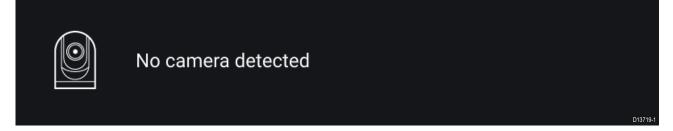
If the '**No camera detected**' message is displayed for more than 2 minutes, then your MFD cannot connect to your camera. Ensure network and power connections to your camera and MFD are correct and free from damage and then power cycle your system. If the camera feed is still not displayed, refer to your equipment's installation documentation for further troubleshooting information.
