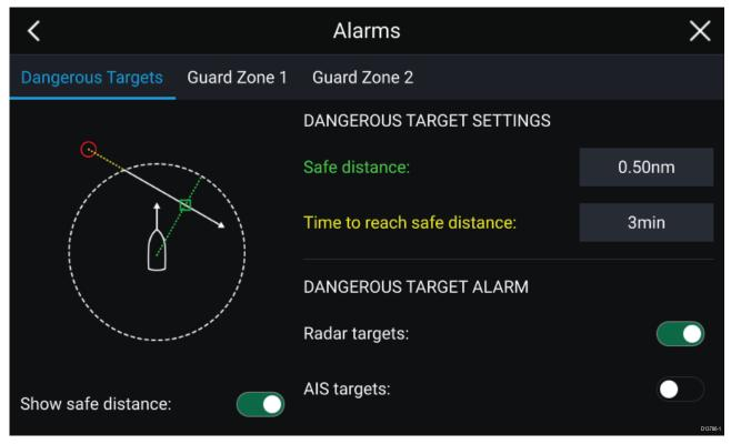
To set up the Dangerous target alarm, first adjust the **Safe distance** to the desired value and then select a **Time to reach safe distance**. The alarm will be triggered if a tracked target will reach the specified Safe distance from your vessel within the time period selected.
