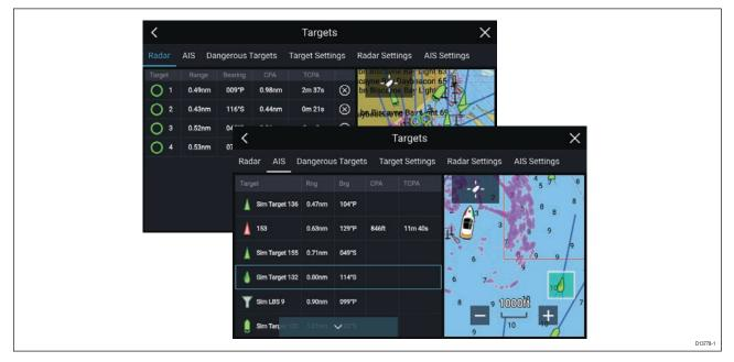
Selecting a target from the list will highlight the selected target in the app pane on the right of the screen.
