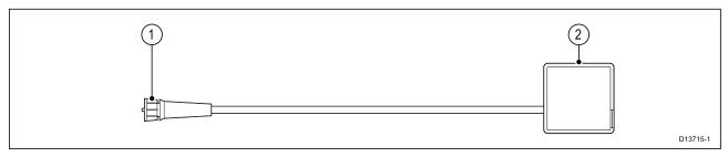
The RCR-SDUSB accessory can provide your MFD with extra storage by connecting external storage devices i.e.:
