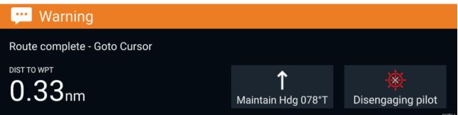
When performing a Goto the Pilot pop-up provides options to disengage the autopilot or to maintain the current course in Locked heading mode.
