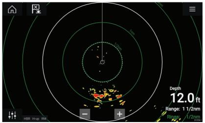
If your Radar scanner is connected, powered up and transmitting then the Radar image is displayed and echoes/targets are displayed onscreen.
