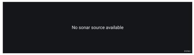
Check your external sonar module's network and power connection, check your MFD's network or transducer connection ensuring the connections and cabling is correct and free from damage, then power cycle your system. If the Sonar module is still not found then refer to your equipment's installation documentation for further troubleshooting information.
