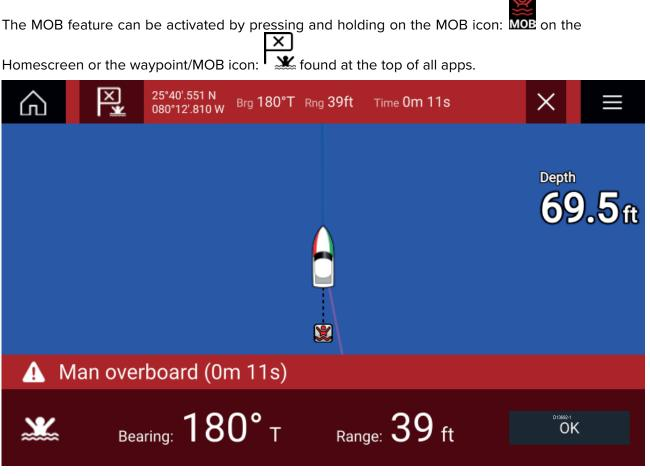
The MOB feature requires your vessel to have a valid position fix from a GNSS receiver. Dead reckoning mode also requires Heading and Speed data.
