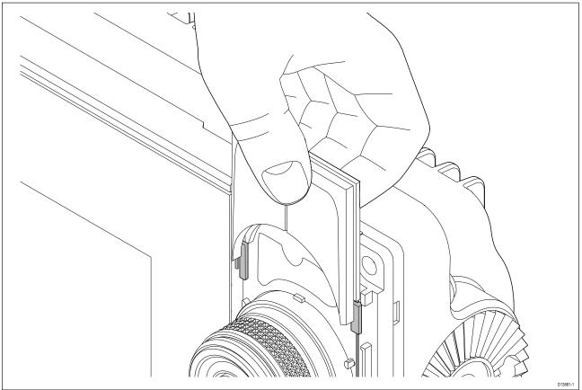
1. Slide the backing plate behind the locating tabs as shown below.
