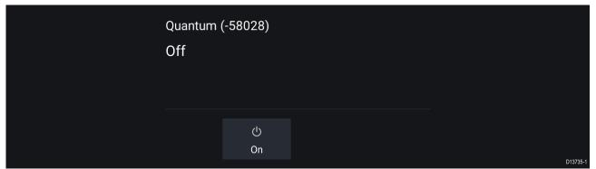
If the '**Off**' message is displayed then your Wi-Fi connected Radar scanner is paired but powered off, select **On** to power up your Radar
