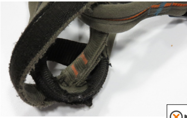
• Worn out belay loop and tie-in point
