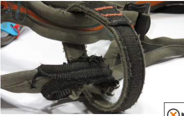
• Worn out tie-in point
