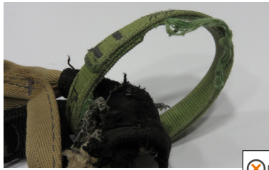
• Worn out belay loop and tie-in point
