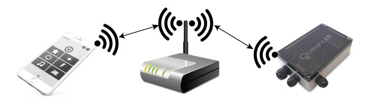
For more advanced users the OceanDMX App controller can also be configured to automatically connect to a local wireless network, allowing phones / tablets to communicate with the controller via the vessels existing Wi-Fi.
