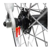
Remove the plastic protection from the lower end of the fork and put the wheel so that it fits. Ensure that the wheel is locked into the fork by making a small force on the handlebar from top to bottom. Tighten the outer axle nut with a 15 wrench or with an adjustable wrench while holding the inner nut with a 17 wrench. You should do the same on both sides.
