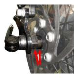
If you want to remove a wheel with quick release system, you should just open the lock and remove the wheel.
