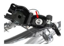
Raise the handlebars and make sure that it has been perfectly aligned. Otherwise, repeat the step.
