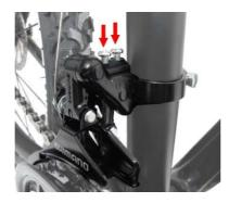
Place the chain and controls on smallestchain wheel and on the largest sprocket. Turn the inner boundary regulating screw (L) so that the chain approaches as much as possible to the left side of the derailleur, but without touching it.
