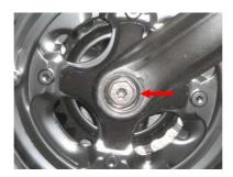
If you want to change a crank arm, loose the screw and remove the crank arm. The bottom bracket has a cone-shape, so that, after a period of use, the crank arms are securely tightened. We recommend using a crank extractor for their removal. Remember that the right crank is part of a larger piece which includes the chain wheels.
