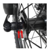
Pass the quick release system inside the axle, by putting it on the opposite side to the disc, and screw the nut (on the side of the disc) giving only a few laps, enough to prevent a fall. Leave the quick release open. This has to go on the opposite side of the brake disc.
