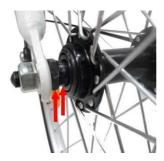
To assembly the wheel, put it in his place, and do the reverse operation: tighten the outer nuts (one on each side), while holding the inner one.
