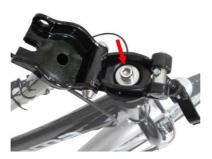
Raise the handlebar and align it with the wheel. Fold downwards the handle and tighten the screw.
