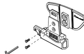
**Step 2.** Tighten the screw plate to the slide-in mounting kit with the two provided screws.
