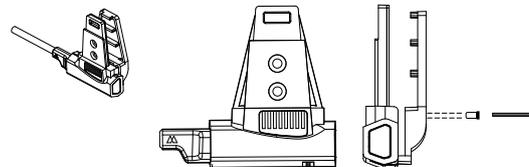
If necessary, you can use also the rubber plate in order to have more grip for the screw clamp. Just use the two short screw to fix the rubber plate on the slide-in mount and tighten the screw plate again.
