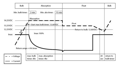
Figure 2. Typical charge characteristic (at 25°C / 77°F). For a 24V charger, multiply the voltages by two.
