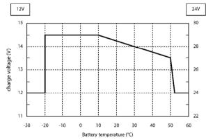
Figure 1. Temperature compensated charging
