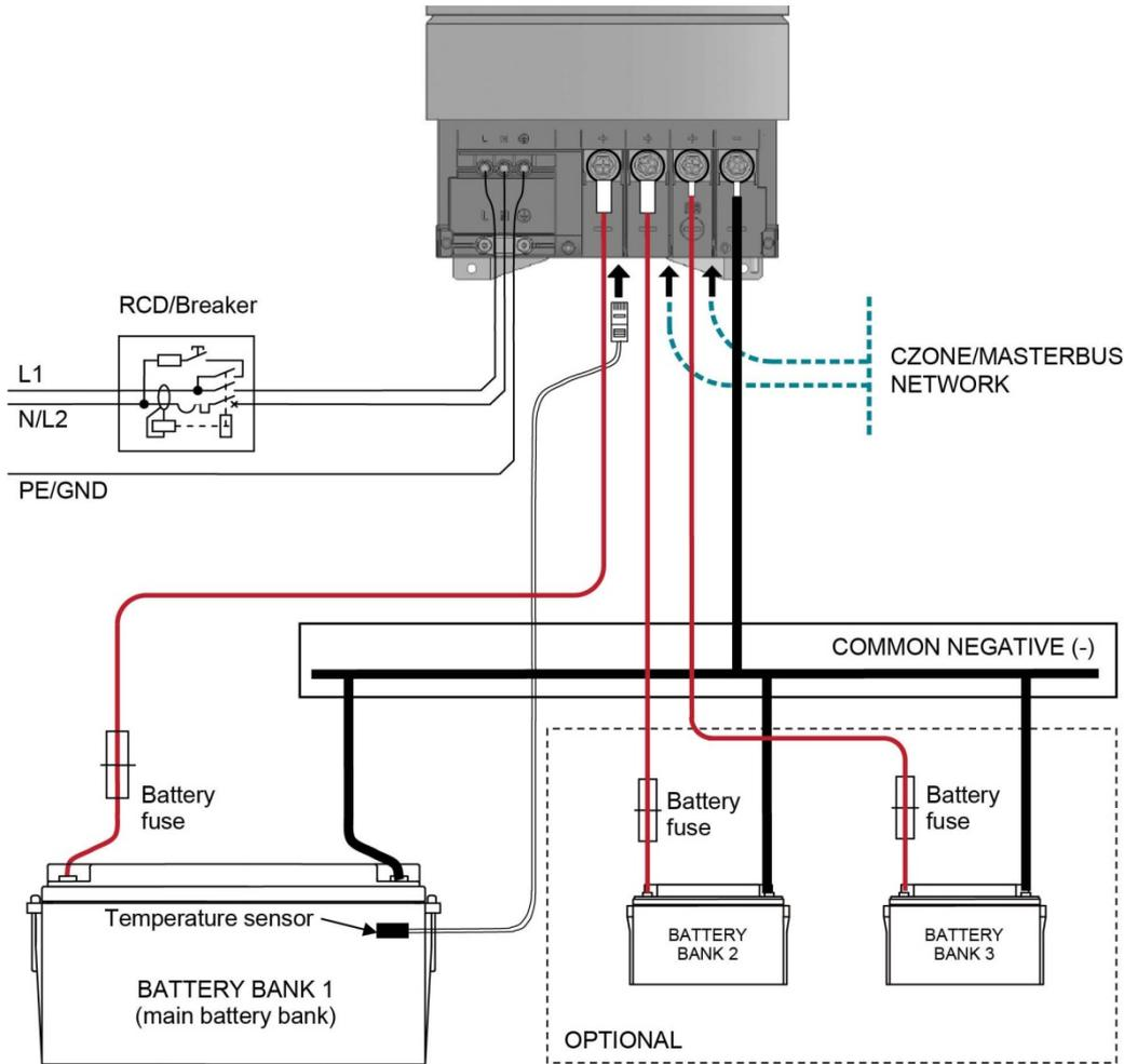
Figure 3: Installation drawing of the ChargeMaster Plus
