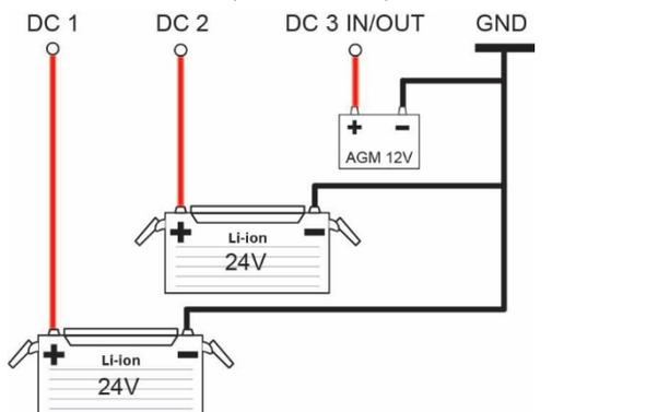
If DIP switch 7 is in the on position, then DC 3 IN/OUT is current limited to 10A to safely charge a small starter battery. When a 24V charger is used, DIP switch 6 can also be in the on position, unless the 24V charger must charge a 24V starter battery.
