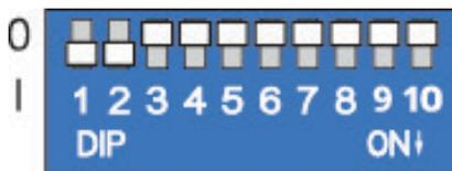
Figure 4: DIP switches (factory settings)
