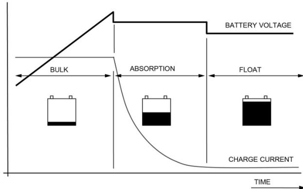
Figure 6: charge process
