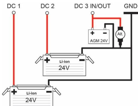
Three full outputs. All batteries are charged with the same settings. DC 3 IN/OUT acts as a VSR (Voltage Sensitive Relay). When there is no AC power available and the alternator is charging the starter battery, the alternator can also be used to charge batteries 1 & 2. The threshold voltage which is used to switch over is set via the configuration tool.
