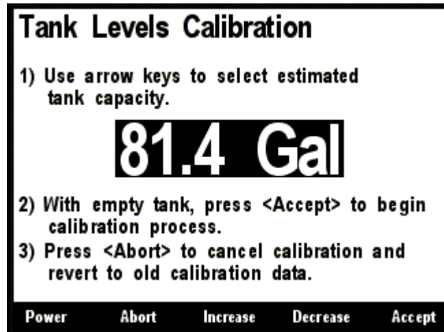
Figure 216 – Tank Levels Calibration Capacity Estimation
