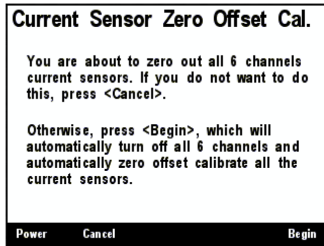
Figure 61 – DCR100 Current Sensor Zero Offset Calibration Screen
