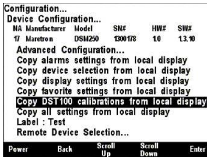
Figure 75 – DSM150/DSM250 Copy DST100 calibrations from local display
