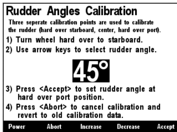
Figure 155 – RAA100 Starboard Rudder Angle Calibration
