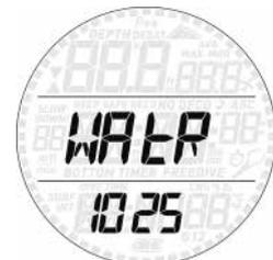
Unlike most scuba and apnea instruments which only allow to choose between fresh water and salt water, in Smart Apnea you can set the water density between 1.000 (freshwater) and 1.050 in 0.001 increments. Default setting is 1.025, which corresponds to the salt water setting in Mares dive instruments.
