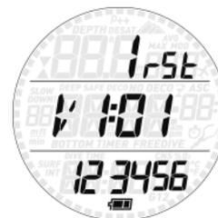
This submenu provides information about the hardware and software of your Smart Apnea and about the status of the battery (two segments inside the battery means the battery is ok, one segment means the battery is low but the watch functions as dive computer, one segment blinking means the battery is too low for use as dive computer).
