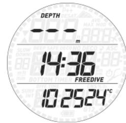
The pre-dive display shows time of day and temperature. The 4-digit number in the bottom left corner is the set water density without the decimal point. Refer to section 2.3.1 for more information about setting the water density.
