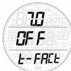
The minimum surface interval is defined as the duration of the previous dive multiplied by the t-factor. The t-factor can be set between 1 and 7 in 0.5 increments.
