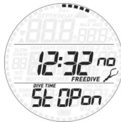
The **pre-dive** mode puts the computer in a ready-to-dive mode and ensures that Smart Apnea starts to monitor the dive as soon as a depth of 1.2m/4ft is reached. If you start the dive without putting Smart Apnea into **pre-dive** mode, it will start to monitor the dive automatically but with a delay of up to 20 seconds from immersion.
