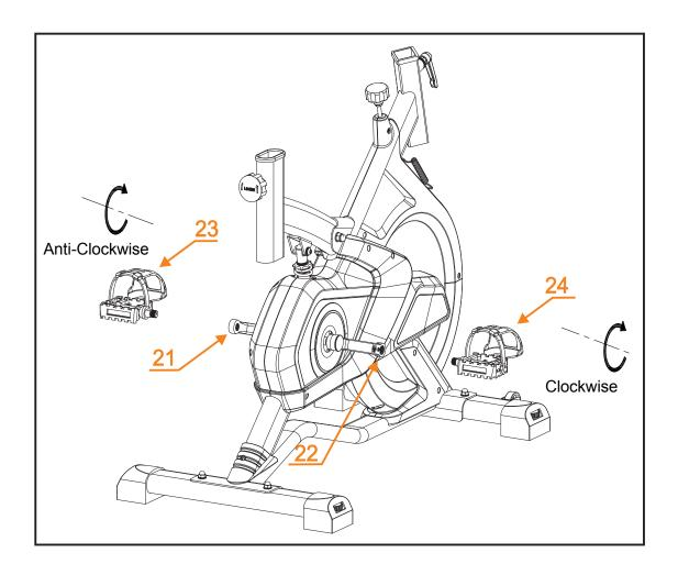
SCREW THE RIGHT AND LEFT PEDAL (23/24) TO THE LEFT AND RIGHTCRANK (21/22).SCREW 4-5 CIRCLES BY HAND, THEN FASTEN IT WITH THE WRENCH.
