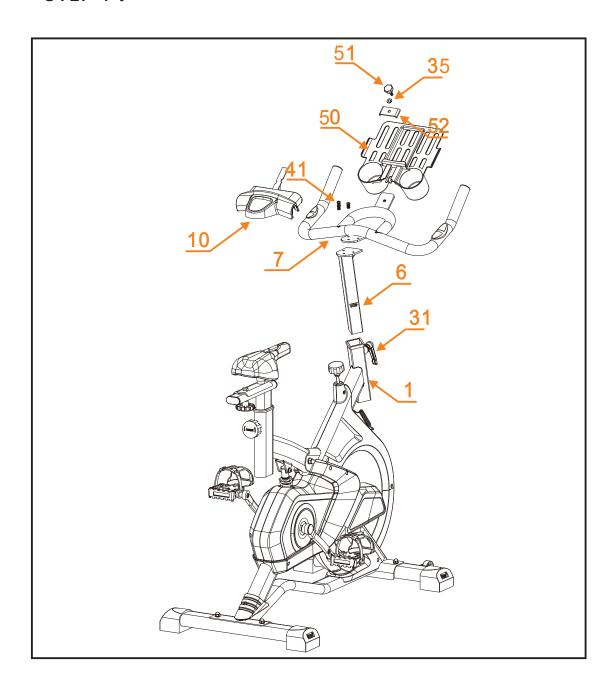
AS THE PICTURE SHOWS, LOOSING NUTS UNDER PHONE CAGE (10) AND REMOVE IT FROM HANDLEBAR (7).
