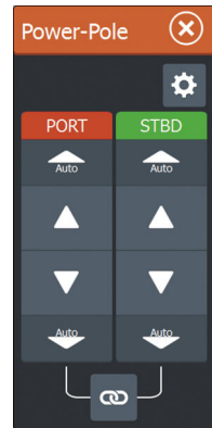
Dual Power-Poles controller
