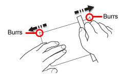
Before loading Hagaki (Cardstock) into the multi purpose tray, fan them and align the edges. If the Hagaki (Cardstock) paper is curled, straighten it before loading. Printing onto curled Hagaki (Cardstock) may cause jams.
