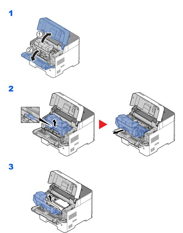
If the jammed paper appears to be pinched by rollers, pull it along the normal running direction of the paper.
