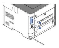
5 Insert the power cord into the socket and turn on the power switch.
