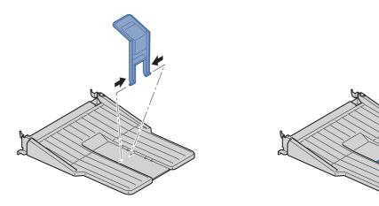
2 Install the rear tray on the rear of the machine.
