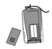
3. Close the battery door completely by reversing Step 1.
