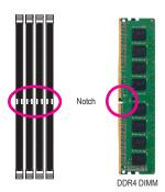
A DDR4 memory module has a notch, so it can only fit in one direction. Follow the steps below to correctly install your memory modules in the memory sockets.
