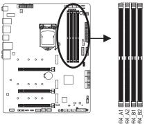
▶ Recommanded Dual Channel Memory Configuration:
