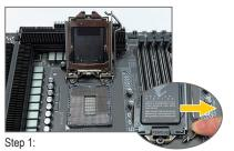
Gently press the CPU socket lever handle down and away from the socket with your finger. Then completely lift the CPU socket lever and the metal load plate/plastic cover will be lifted as well.
