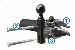
**NOTE:** both 1/4 in. (65 mm) standard and M6 bolts are included. Match the size of the factory bolts on your clutch-clamp or brake-clamp bracket.
