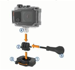
3 Allow the base to bond to the mounting surface for at least 24 hours.
