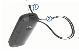
2 Thread the other end of the lanyard ② through the loop, and pull it tight.
