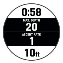
**In-dive screen**: Displays the information about the current dive, including the elapsed time, current and maximum depth, and rate ascent or descent. You can edit the data screen layout and data fields (*Customizing the Data Screens*, page 99).
