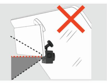
**3** After you have selected a mounting location with a clear view, remove the protective film from the mount adhesive.
