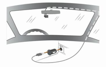
The shorter cable is designed to be routed down to your vehicle power supply.
