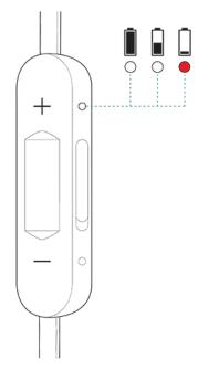
While Flyer is on, check the current battery level at any time by briefly pressing the Power button.
