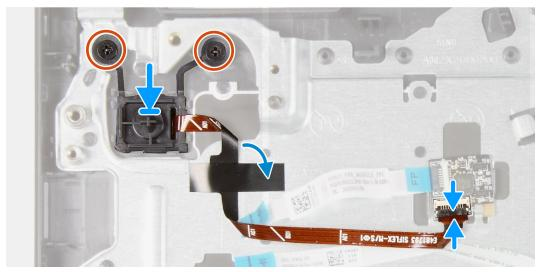
NOTE: When replacing/re-installing the power button with fingerprint reader assembly on the Vostro 3501, a mylar sticker must be adhered to the fingerprint reader FPC to ensure that it is properly grounded to the palm rest. The mylar sticker is packaged together with new replacement power button with fingerprint reader assemblies
