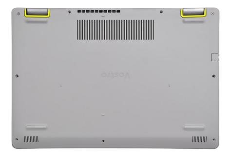
NOTE: CAUTION: DO NOT pry up from the edge near the vents at the top side of the base cover as this may damage
