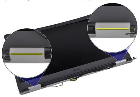
4. Pry open the display bezel from the inner edge at the bottom side of the display assembly.
