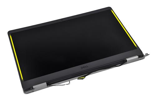
2. Pry open the display bezel from the inner edge at the top side of the display assembly.
