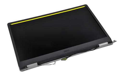
${\bf 3.}\;\;$  Pry open the hinge caps at the bottom side of the display assembly.
