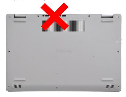
**3.** Lift up the top side of the base cover and remove it from the system.
