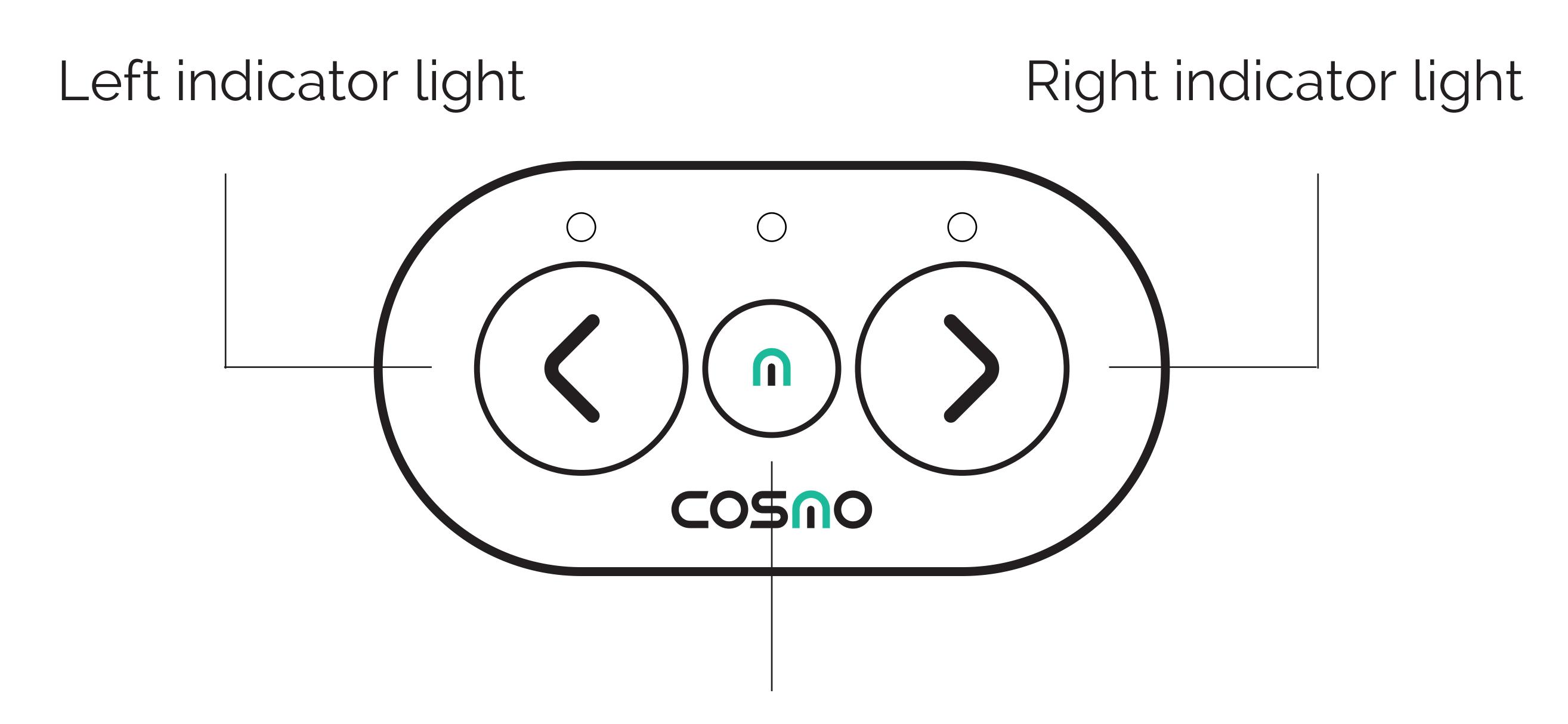
Middle button: hold down to turn off the Cosmo Ride or press quickly to change the lighting mode. There is one return light per light mode (details below mode 1, 2, 3, 4)
