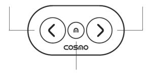
Middle Button: long press to switch off the Cosmo Bike or short press to change ignition mode (detail below mode 1,2, 3, 4)
