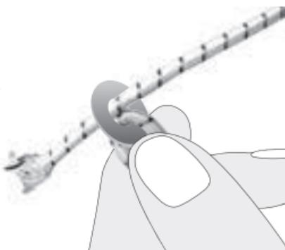
3. Knot both ends of the elastic and adjust to ski tip, then tighten the knots.
