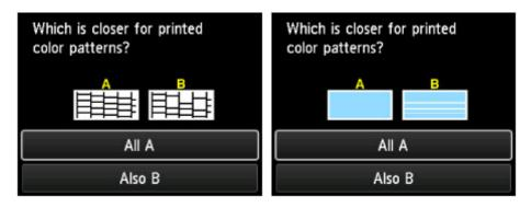
If pattern C has no missing lines in all three groups and pattern D has no horizontal streaks (A):
