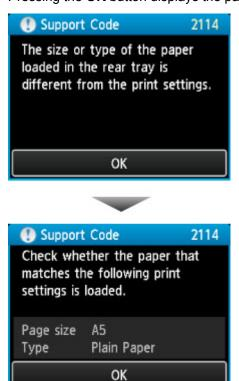
Check the message and press the **OK** button. When the screen to select the operation is displayed, select one of the operations below.
