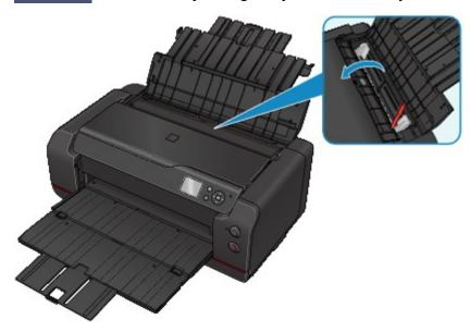
If there are any foreign objects in the rear tray or the manual feed tray, be sure to turn off the printer, unplug it, and then remove the foreign object.
