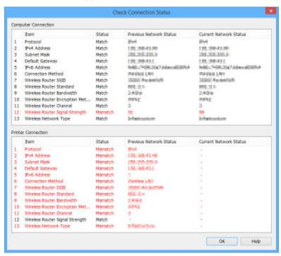
If the network status when you used the printer is different from the current status, **Mismatch** appears on **Status** and the items are displayed in red. Check the red items.
