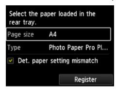
Select **Register** and press the printer's **OK** button to finish setting the rear tray paper settings.
