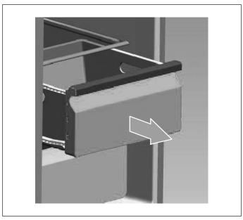
To insert the container, place on the telescopic rails and push into the appliance. Attach the container by pressing it down.
