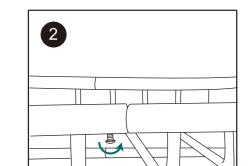
Then secure it with machine screws by provided wrench.
