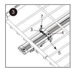
Now lock the saddle (3) onto basket. The saddle must sit on the cross bar then secure it with bracket top plate (4), bracket plate (5), and choose the bolt with appropriate length, 65mm (7) or 50mm (9) M6 screw are available, so that they will not damage the car roof.
