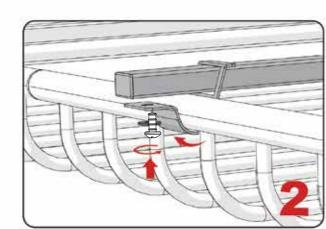
Fix the bracket by tightening the bolt with nut provided. Follow the same steps at both sides. 依序將輔助桿鎖固於行李盤的兩側。
