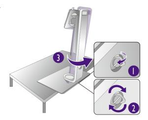
Gently turn the screen over to install the monitor stand arm and base.
