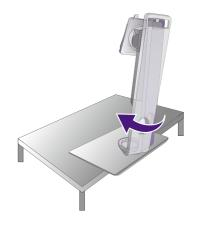
Tighten the thumbscrew on the bottom of the monitor base as illustrated. And then turn the stand counterclockwise to face forward.
