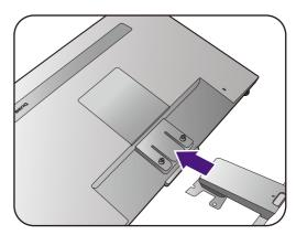
Tighten the screws that fix the stand to the monitor.
