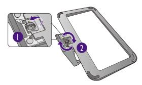
Orient and align the stand arm with the monitor, then push them together until they click and lock into place.
