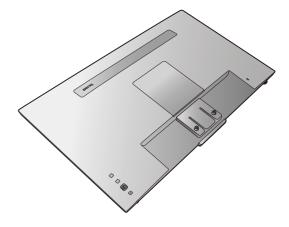
Attach the monitor stand to the monitor base as illustrated until it locks in place.
