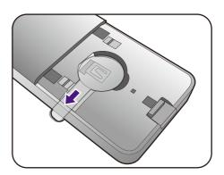
4. Replace the provided battery (CR2032) onto the battery holder properly. Make sure that the positive terminal (+) faces upward.
