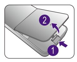
2. Press down the upper part of the battery so you can remove the battery from the lower part as illustrated.
