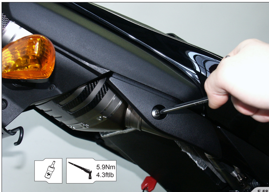
14. Position of the correctly installed Akrapovic SLIP-ON system (F 59).
