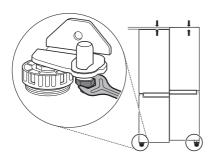
1 Open the door and use the spanner • to loosen the keeper nut by turning it to the left.
