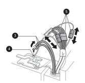
4 Rotate the hinge lever **3** counterclockwise. Lift the top hinge **9** free of the hinge lever latch **3**
