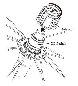
4. Tighten the adapter with the lockring tool and torque wrench .The tightening torque is 40 N-m.
