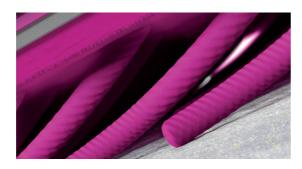
During the manufacturing process of POMOCA's GLIDE equipment, the entire length of the skin's fibers is subjected to a chemical treatment to reduce the friction on each of the fibers so that even crystals in virgin snow won't stick to them. At the same time, the skin's surface is permanently protected.
