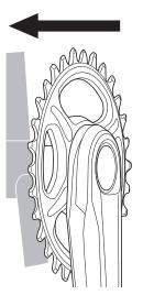
**2.** Completely tighten the adjustment nut of the left crank arm.
