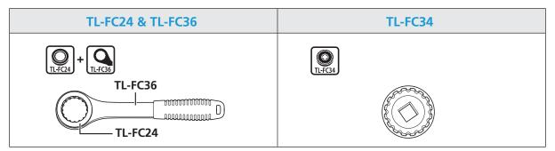
Installing/removing the bottom bracket
