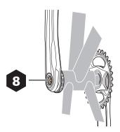
**2.** Remove the right crank arm unit from the bottom bracket.
