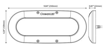
${\rm NOTE:}$  When installed for DMX use, light cables cannot be extended further than the supplied 3m between junction box and light.
