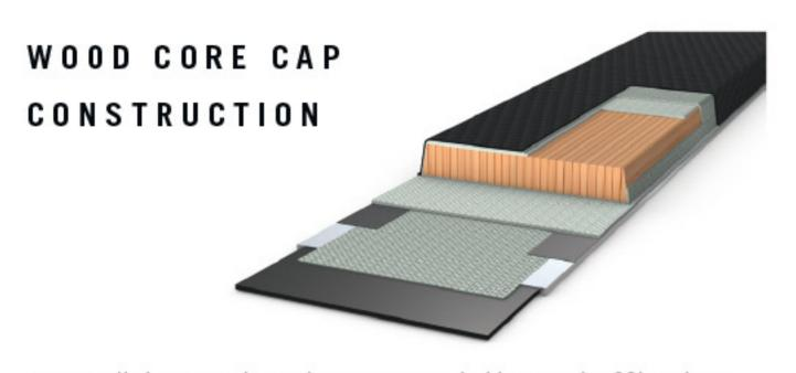
A vertically laminated wood core surrounded by a sock of fiberglass and the whole body is wrapped by a durable topsheet. This forgiving construction is ideal for ramping up the learning curve.
