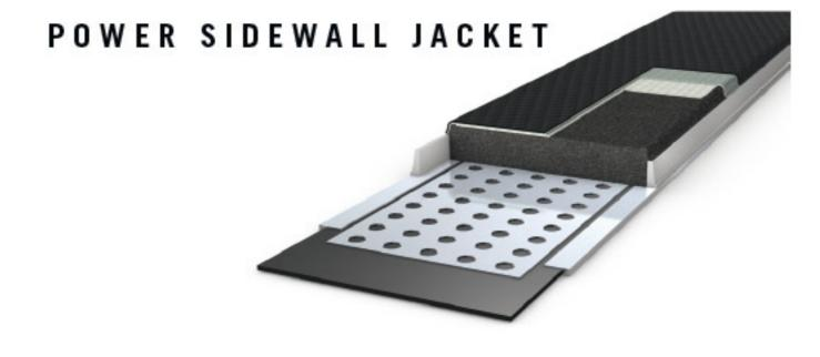
A synthetic injected core supported with ABS sidewalls. This lightweight construction allows for a soft longitudinal flex coupled with a super responsive torsional flex, thanks to the sidewall Jacket.
