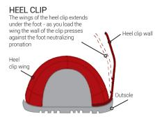
When the foot pronates load is applied to the wing
