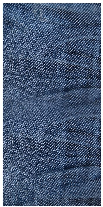
Aramid fibre with very high tensile strength, tear, cut and heat resistance, together with low electrical conductivity and excellent resistance to chemical agents. Optimal mechanical performance combined with light and soft yarn guaranteeing both comfort and fit.
