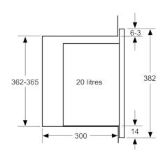
measurements in mm
