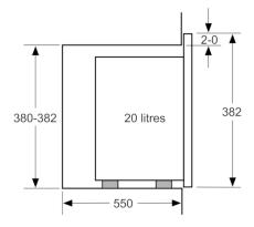
measurements in mm
